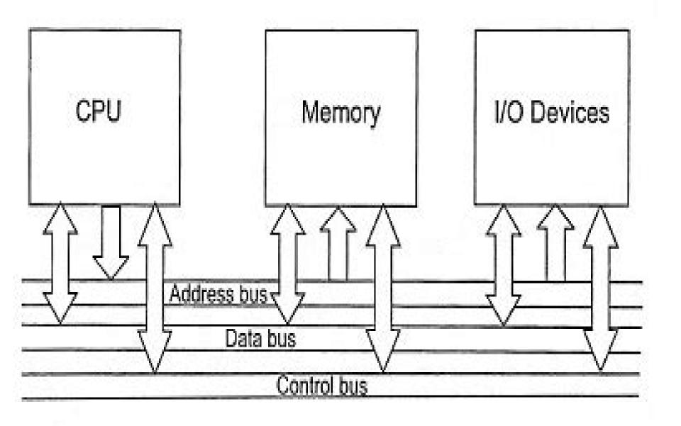
Fig. 9.67 Bus structure of a microcomputer
