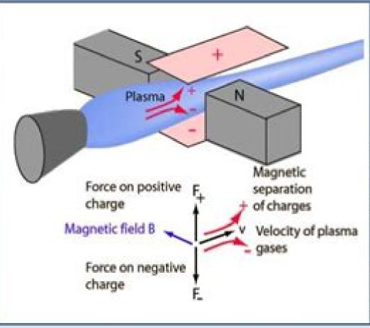
Magnetic Field Perpendicular Current Magnetic Fluid Magnetic metals ·Plasmas ·Salt water The idea of MHD is that magnetic fields can induce currents in a moving conductive fluid, which create forces on the fluid. The set of equations which describe MHD are a combination of the Navier-Stokes equations of fluid dynamics and Maxwell's equations of electromagnetism.
