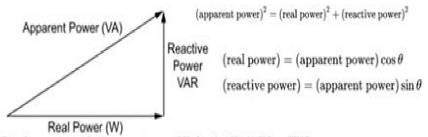
Real power = Active power = VI Cosθ, Unit W or KW Reactive Power = VI Sinθ, Unit VAr or KVAr Apparent Power = VI, Unit VA or KVA
