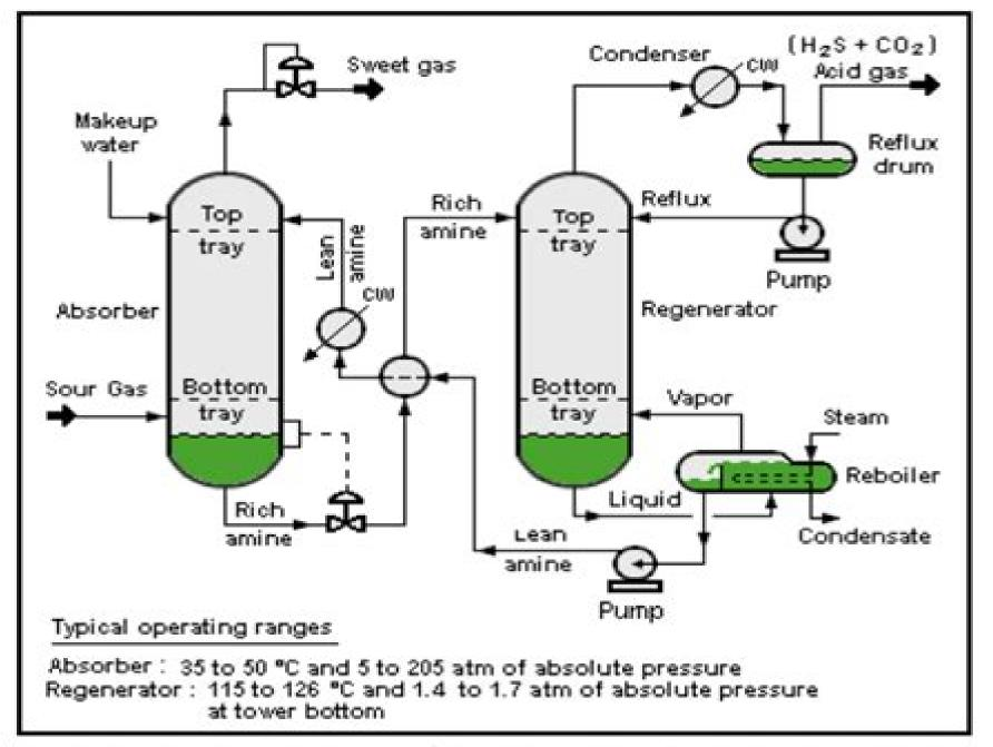
Figure 1: Example of a process simulation model
