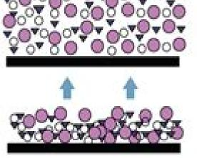
Dry Coating Film Pignent Particles and Binder Huse Together and Create a Continuous Film
